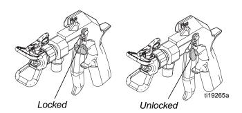
Fig. 1: Trigger Lock Positions
