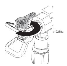
Spraying position shown. Rotate tip handle 180° and trigger gun to clear clog.
