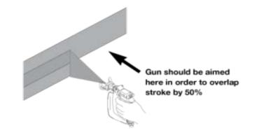
• The applicator should spray with an "X" out technique, 2 light passes at once (wet on wet) with one pass side to side and the next pass up and down. This technique helps to ensure a uniform coverage over the sometimes uneven surface of the SPF. Passes should not be confused with coats which require 4 hour dry time in between as opposed to a wet on wet pass.
