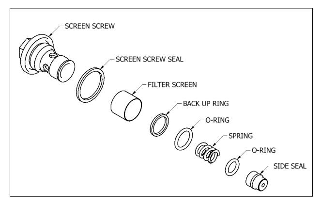
**CAUTION!** To avoid possible contamination by the residual chemical inside the Gun do not interchange the Isocyanate (A) parts with the Polyol (R) parts. The Isocyanate (A) side is identified with an (A) on the Screen Screw Head and the Polyol (R) side is marked with an (R) on the Screen Screw Head. The Gun Block is also marked with (A) and (R) designation.
