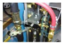
5. Check pump lube. If lube is milky in color, or not clear, dispose and refill lube jar 3/4 full.
