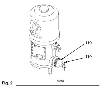
In a direct supply system, with adequate air pressure supplied to the motor, the pump starts when the gun or dispensing valve is opened, and stalls against pressure when it is closed.
