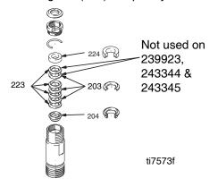
5. Install seal (201) into packing nut (202). Install throat adjustment spacer onto packing nut. Loosely install packing nut into cylinder.
