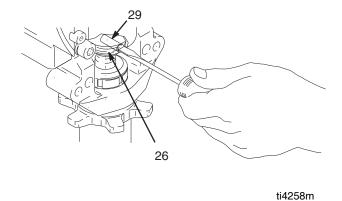
23. Reassemble intake valve with new o-ring (227), seat (212) and ball (204). Seat may be flipped over and used on other side. Clean seat thoroughly.
