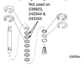
15. Soak all leather packings in SAE 30W oil for 1 hour minimum prior to assembly. Stack male gland (219) on piston rod. Alternately stack UHMWPE (208) and leather (218) packings (note orientation) on piston rod. Install female gland (217). Install backup washer (216) and u-cup (209) (note orientation) on piston valve (210). The special sealing patch on piston valve threads is good for four repackings. Use thread sealant on piston valve threads after four repackings.
