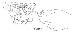
13. Soak all leather packings in SAE 30W oil for 1 hour minimum prior to assembly. Stack male gland (204). Alternately stack UHMWPE (203) and leather (223) packings (note orientation). Install female gland (224). Install seal (201) and packing nut (202) and throat adjustment spacer (228).
