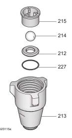
11. Install intake valve on cylinder. If a wrench is used torque as follows:
