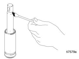
9. Grease o-rings (221) and place on sleeve. Slide sleeve/piston rod assembly into bottom of cylinder. Replace o-ring (207) if desired. **NOTE:** O-ring (207) is not required for safe pump operation.
