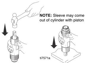
Remove piston rod from sleeve, or remove sleeve from cylinder. Remove o-ring (221) from top of sleeve (or from inside of cylinder if o-ring did not come out with sleeve).
