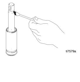
20. Grease o-ring (221) and place on sleeve. Slide sleeve/piston rod assembly into bottom of cylinder. Replace o-ring (207) if desired. NOTE: O-ring (207) is not required for safe pump operation.
