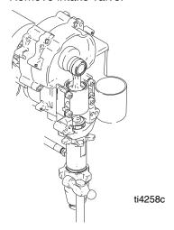
3. Use screwdriver to push retaining spring (26) up.
