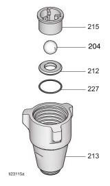
24. Install intake valve on cylinder. Torque as follows:
