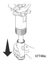
7. Invert piston rod and sleeve and pound on hard surface until piston rod comes out of sleeve.
