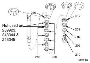
16. Install ball (206) in piston rod. NOTE: If thread sealant is applied to piston valve threads, make sure none gets on ball. Install piston valve on piston rod. Torque as follows:
