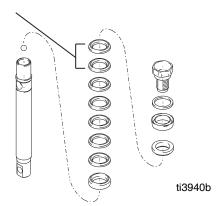
8. Remove throat packings and glands from cylinder. Discard throat packings and glands.
