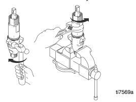
Disassemble intake valve. Clean and inspect o-ring (227). NOTE: A pick may be required to remove o-ring.
