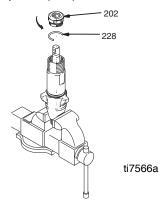
2. Unscrew intake valve from cylinder.
