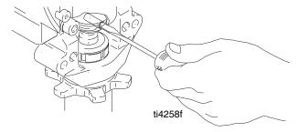
11. Remove piston valve from piston rod with a wrench.
