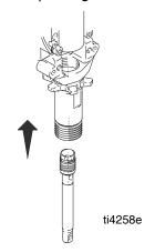
Insert piston rod into cylinder with pin hole up and piston valve down. Insert pin into piston rod and crank shaft.
