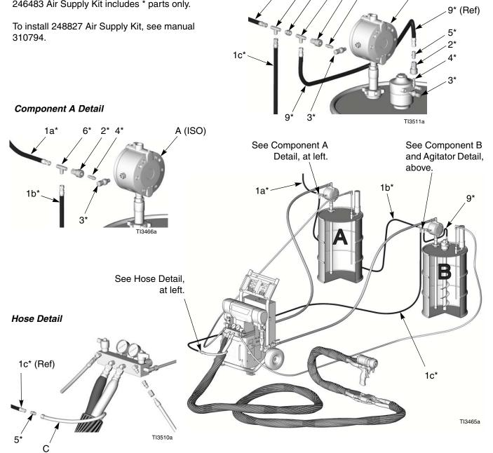
Component B and Agitator Detail
