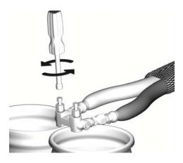
FIG. 13: Open Manual Valves
