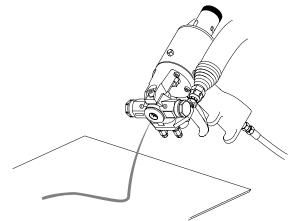
4. Release gun trigger, CLOSE safety stop, and close manual valves.
