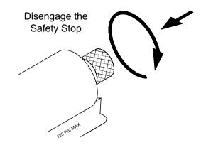
FIG. 5: Safety Stop - Disengaged
