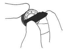
FIG. 19: Unthread Cap from PCD Body
