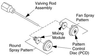
FIG. 3: Mixing Module & PCD
