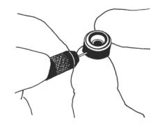
FIG. 20: Clean Module Ports
