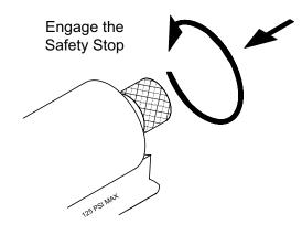
FIG. 4: Safety Stop - Engaged
