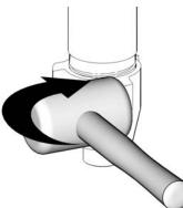
12. Torque packing nut (202) down to 50 ft-lb (68 N•m).
