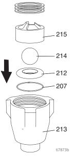
Place intake valve (213) assembly in vice. Install cylinder (205) assembly to intake valve. Torque to 350 ft-lb (475 N•m).
