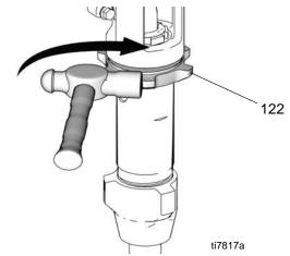
15. Install coupling (125) around pump rod.
