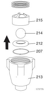
3. Select proper ball travel for material sprayed. Reas semble as shown.
