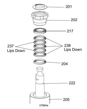
10. Reassemble intake valve (213) as shown.
