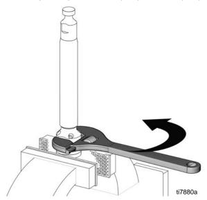
4. Remove parts. Note orientation of parts for reas sembly.
