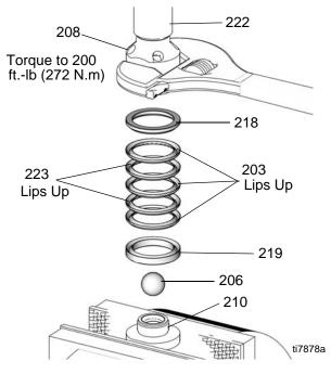
3. Grease piston rod (222) packings and top edge of sleeve (220).
