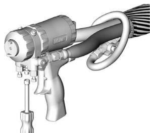
3. Adjust the gun air regulator on the proportioner control panel to desired gun air pressure. Do not exceed 130 psi (0.2 MPa, 2 bar).
