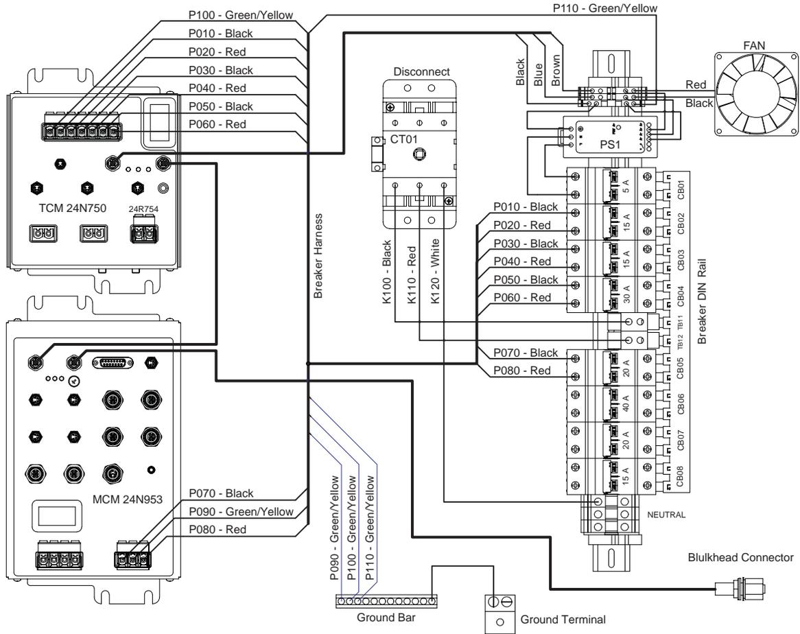
Figure 13 Circuit Breaker Connections Inside Electrical Enclosure (DB)
