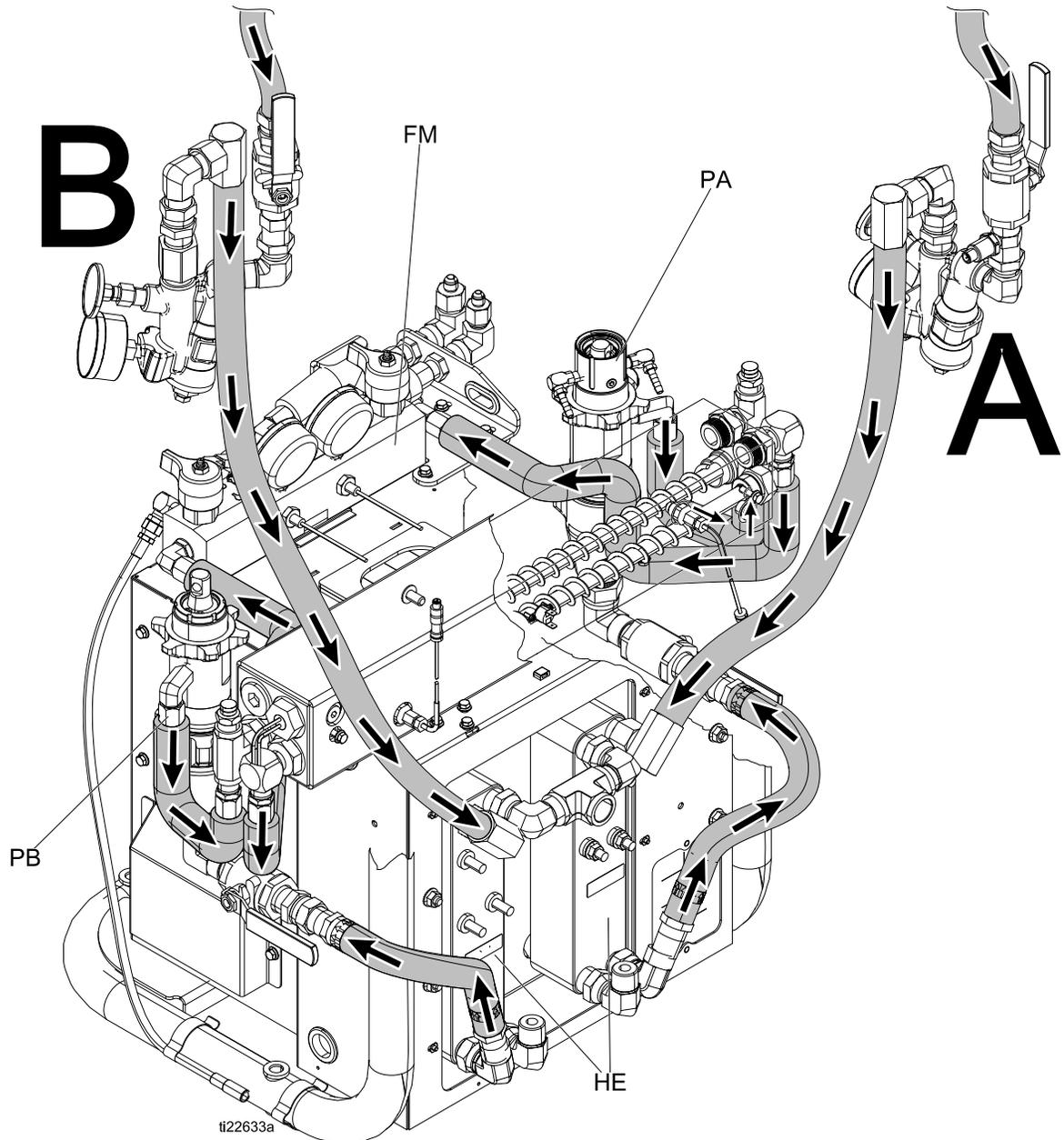
Figure 17 A and B Component Material Flow
