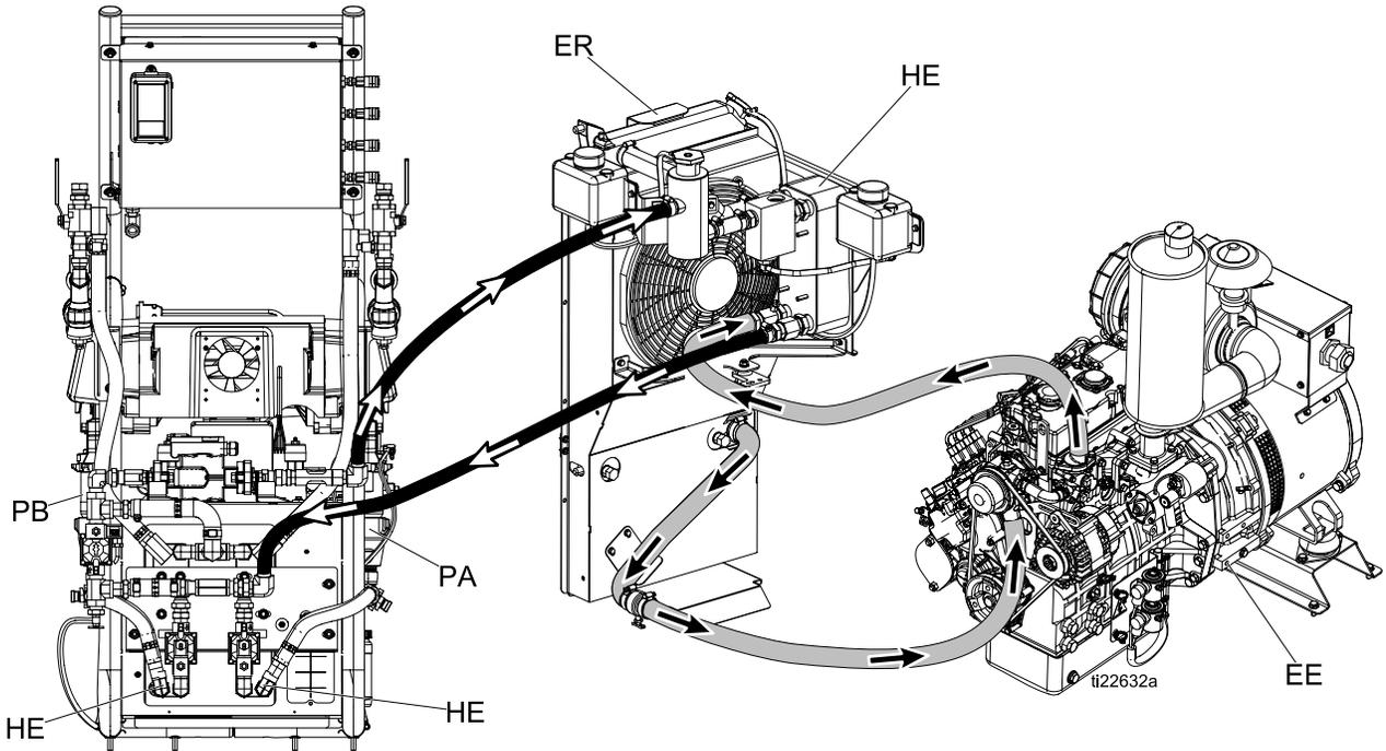
Figure 16 Engine Coolant Loop and Proportioner Coolant Loop
