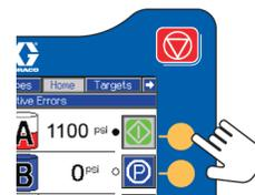
9. Check fluid pressure gauges (GA, GB) to ensure proper pressure balance. If imbalanced, reduce pressure of higher component by **slightly** turning PRESSURE RELIEF/SPRAY valve for that component toward PRESSURE RELIEF/CIRCULATION
