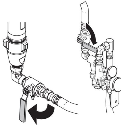
12. Engage gun piston safety lock then close fluid inlet valves A and B.
