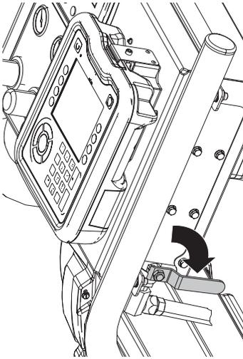
9. Turn main power switch OFF. Allow engine cooling dwell time prior to shutting down the engine.
