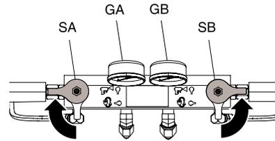
To flush entire system, circulate through gun fluid manifold (with manifold removed from gun).
