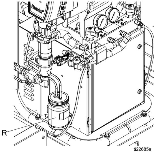
Figure 29 Component A Pump
