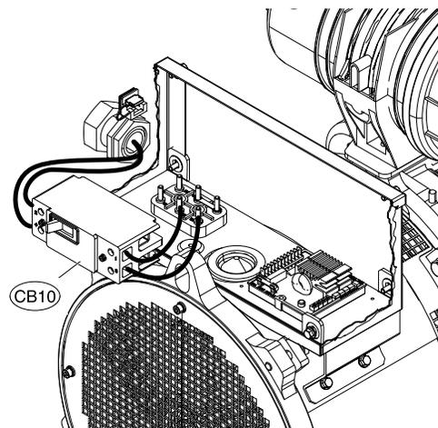
Figure 15 Circuit Breakers Inside Alternator Assembly
