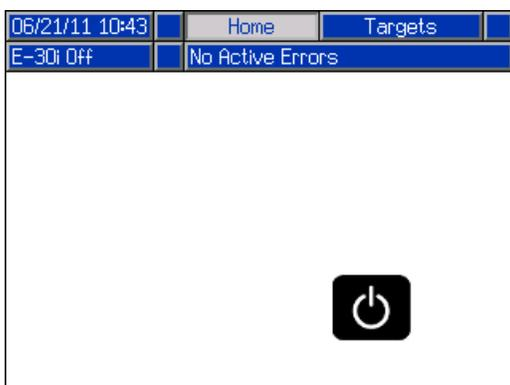
3. Verify the machine is active and the System Status LED is illuminated green, see [Advanced Display Module \(ADM\), page 21](#). If the System Status LED is not green, press the ADM Power On/Off (A) button
